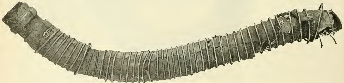
Exterior view of wire-wrapped hose made by a competing company; was on rear of tender of engine. Shows the hose badly burned and burst. Principal cause—wire wrapping and cheap material.
